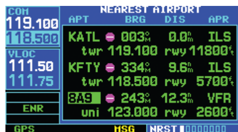
Figure 8-11 Frequency Moved to Standby Field
