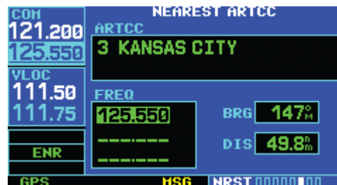
Figure 8-24 Frequency Moved to Standby Field
